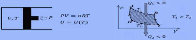
One Carnot cycle consists of four consecutive thermodynamic processes, which can be realized with an arbitrary working substance. We shall consider here however the case of an ideal gas.
